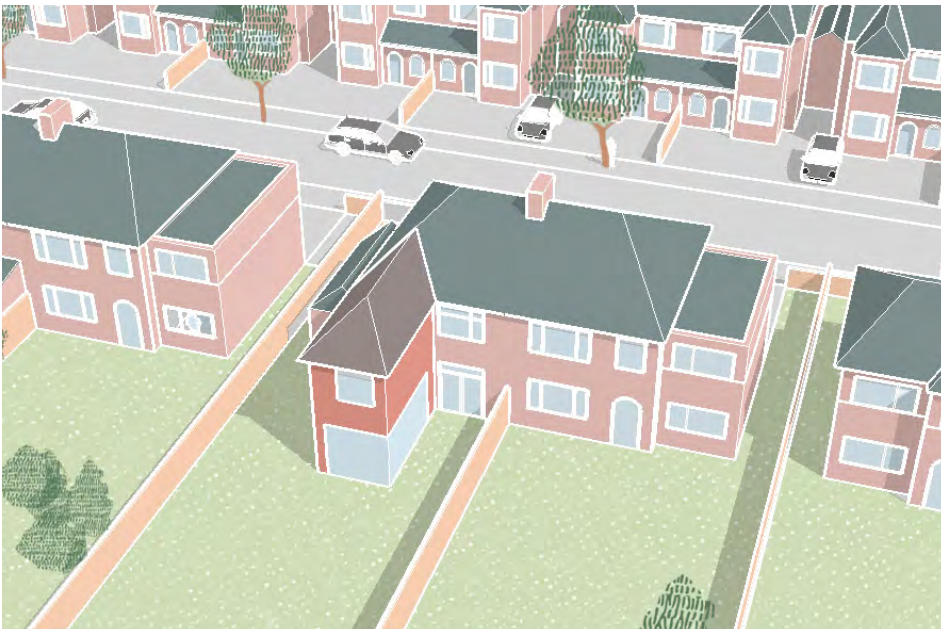
Figure 4.16e: A two-storey extension to a semi-detached house set away from the directly adjoining neighbour.
