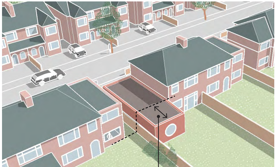
Figure 4.12a: A single storey side extension that extends beyond the rear elevation of a property.
