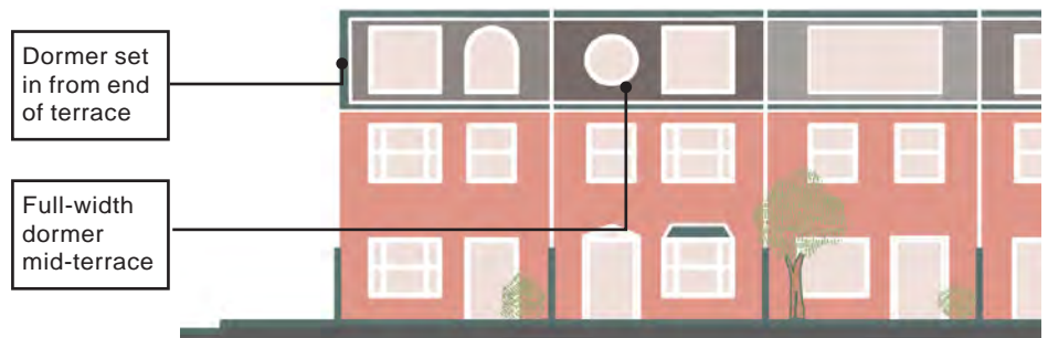
Figure 4.21b: Dormers on a terraced houses that are full-width for mid-terrace houses, but set in from the edge of a gable end (or hipped roof) on the end of terrace house.
